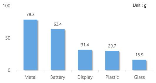
X Calculated the Top 5 heaviest materials of the target model
